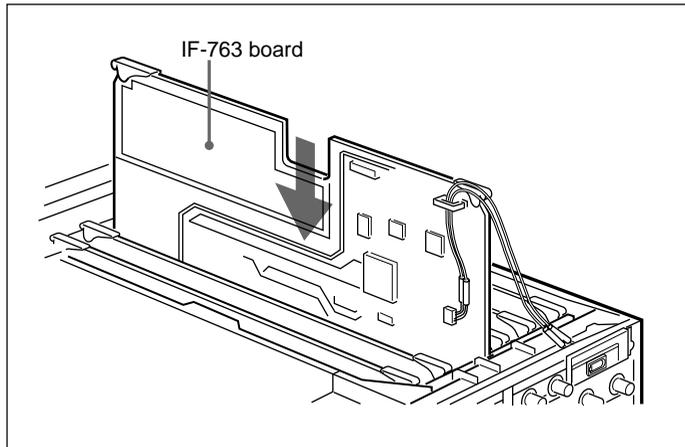
**7** Fix the harness in the cable holder by the board slot.
